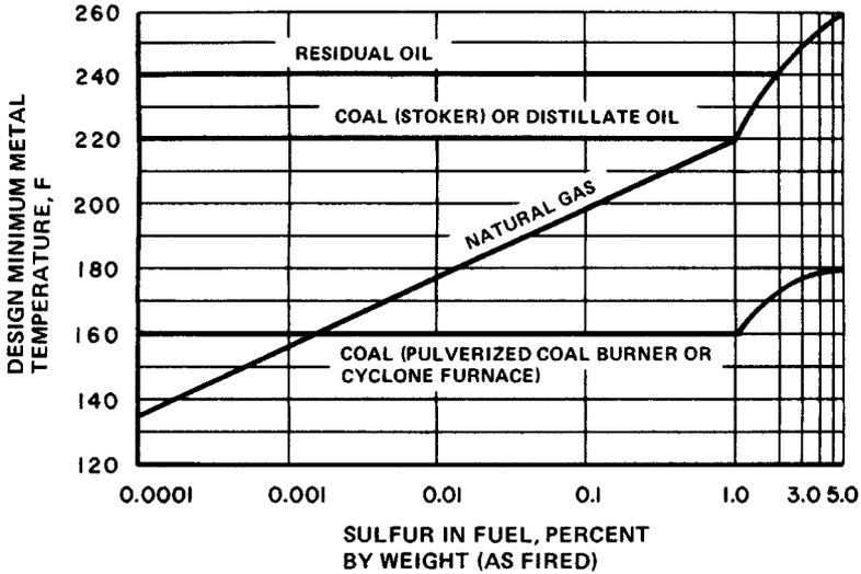
Fig. 53.1 Recommended minimum temperatures to avoid "acid rain" in heat exchangers.
