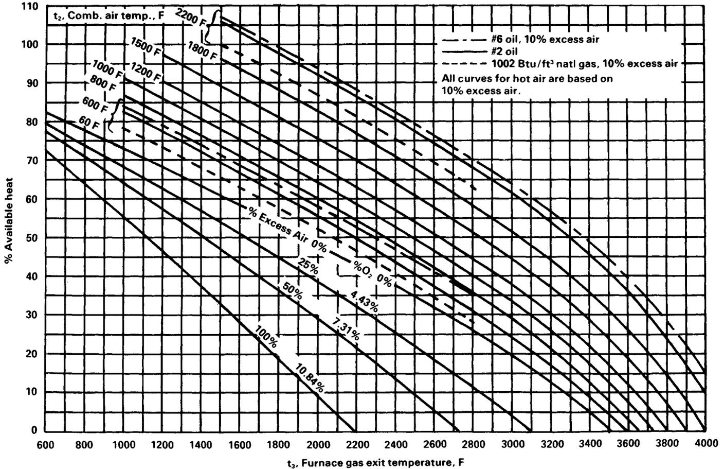
**Fig. 53.2** Available heat with preheated combustion air at 10% excess air. Applicable only if there is no unburned fuel in the products of combustion. Corrected for dissociation. (Reproduced with permission from *Combustion Handbook*.<sup>3</sup>) See also Figs. 44.3 and 44.4.
